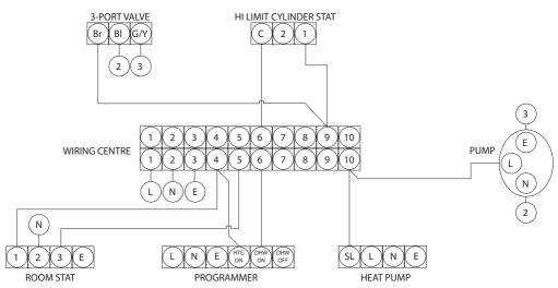
If the 3-port valve itself has not been fitted to building regulations to isolate the heat source from the unvented hot water tank in event of failure, a safety 2-port valve MUST be fitted on the flow into the cylinder coil and controlled via the high limit thermostat provided in the unvented kit, example wiring diagram for this is seen opposite.
